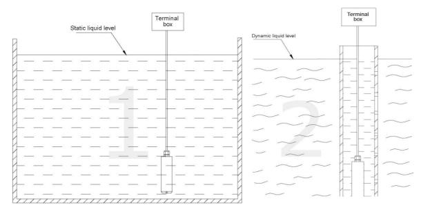
As shown in picture 1, when the sensor is installed in static water such as in poos, water towers, probe is immersed into the bottom and should be as far as possible away from the pump or valves. The terminal box should keep above water surface and prevent water penetrating into cables. Please make sure the airway not be blocked.
