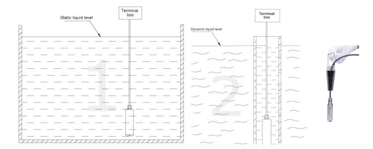
As shown in picture 1, when the sensor is installed in static water such as in poos, water towers, probe is immersed into the bottom and should be as far as possible away from the pump or valves. The terminal box should keep above water surface and prevent water penetrating into cables. Please make sure the airway not be blocked.
