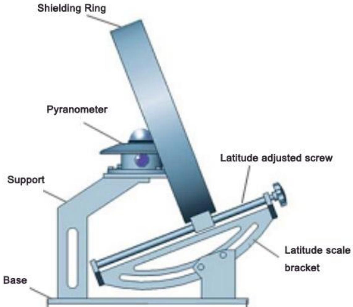
1. First installed Shielding Ring in the observatory, the of the direction and level of shielding ring is important. Therefore, must make the edge chassis when installed on the north and south, make the instrument ruler points to the north and south, (the northern hemisphere, shielding ring handle screw knob toward the north; and the southern hemisphere, south block ring screw adjusting knob handle). Then, the base plate of shielding ring is fixed on the observation bracket with bolts.
