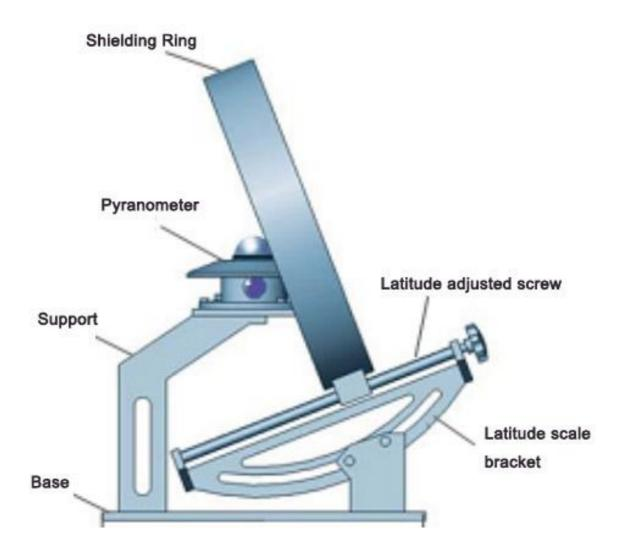
1. First installed Shielding Ring in the observatory, the of the direction and level of shielding ring is important. Therefore, must make the edge chassis when installed on the north and south, make the instrument ruler points to the north and south, (the northern hemisphere, shielding ring handle screw knob toward the north; and the southern hemisphere, south block ring screw adjusting knob handle). Then, the base plate of shielding ring is fixed on the observation bracket with bolts.
